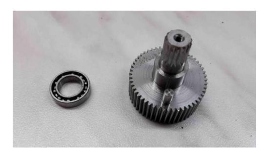
Now comes the real work: removing the pin from the large gear.
