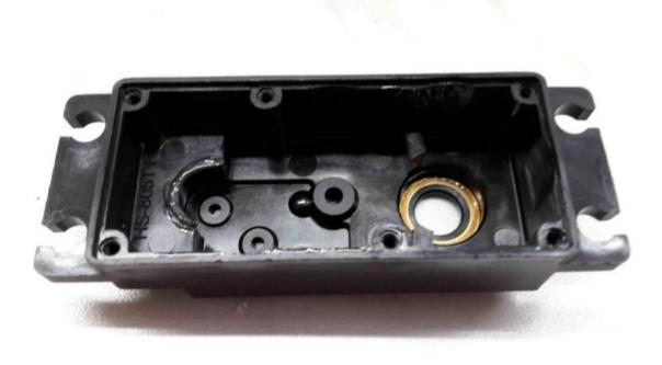
Then carefully pull all the gears off the axles until your servo looks like this. Store the gears dust-free on a clean surface.
