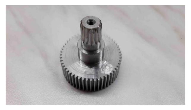
When you are done, thoroughly clean the cogwheel of any sawing or grinding residues. Put the two ball bearings back on both sides of the large gear and reassemble the entire servo in reverse order.
